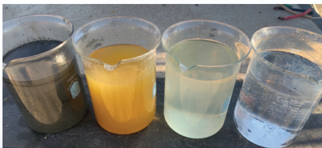
Figure 38: Produced water through our industry partners treatment system, yielding a quality treated water that allows use in our completion operations.
