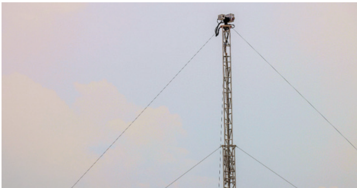
Figure 32: A close-up shot of LongPath's Continuous Open-Path Sensor, which utilizes invisible, eye-safe long-range lasers to detect methane-specific greenhouse gas molecules up to a 2.5-mile radius of installation.
