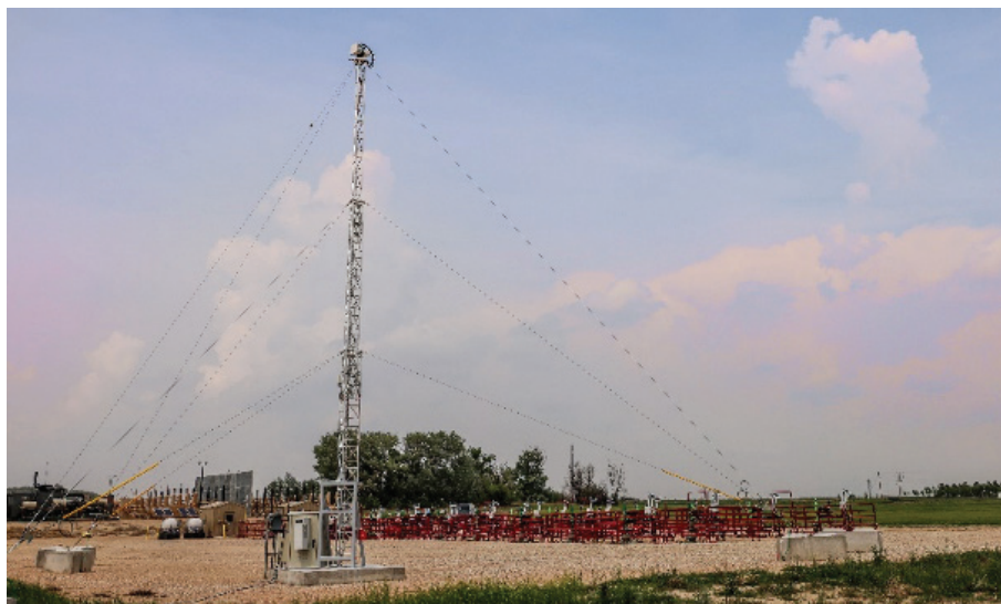
Figure 31: A LongPath sensor located on a Bayswater production site in the DJ Basin.
